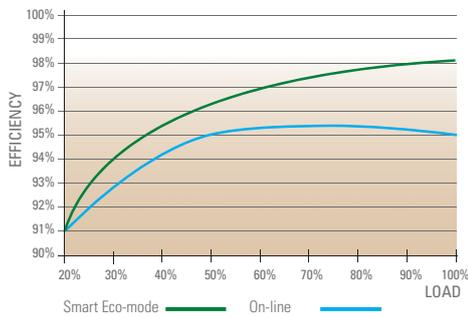
High performance both On-line mode (between 95% and 96%) and Smart Eco-mode (>98%), reducing operating costs, implementation costs (no need to oversize the wiring), air conditioning costs (without increasing cooling requirements) and working costs (saving energy consumed).
