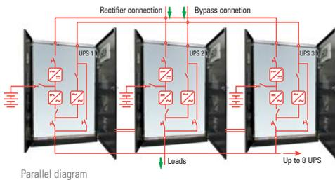
The parallel UPS can be configured to achieve redundancy or increase the power capacity of the system. Parallel control is fully digital and works for active as well as reactive power in each phase, achieving an exact load distribution between the UPS units in transitory conditions.
