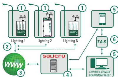
1. Lighting Control Centre: **ILUEST+** with a SICRES card and GSM/GPRS modem.
