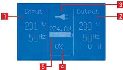
1. Input voltage x phase and frequency.
